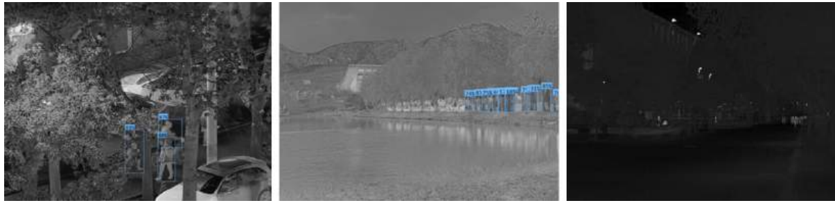
(a) Lower accuracy in highly obstructed environments (b) Decreased performance in crowded environments (c) Reduced system's accuracy on low-quality input images
