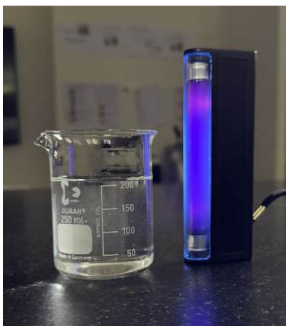
Figure 2. A beaker containing 220 ml of water, exposed to UV light lamp ( \lambda = 254 \text{ nm} ). No fluorescence observed due to absence to UV-active components in solution.
