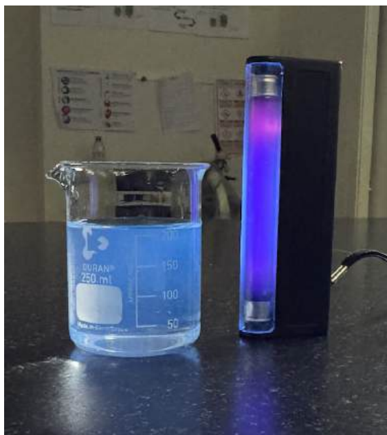
Figure 3. A beaker containing 220 ml of aqueous solution after Horse Chestnut Tree branch stirred, exposed to a UV light lamp ( \lambda = 254 \text{ nm} ), showing blue fluorescence indicating the presence of Aesculin.
