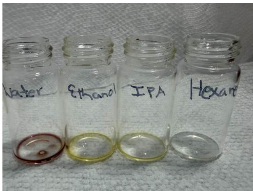
Figure 1. Beet extraction using various solvents. This figure shows extraction of beet using water, ethanol, isopropyl alcohol, and heptane. Water being the most polar solvent and heptane being the least polar. Since ethanol is more polar than IPA, it shows darker yellow due to having a bit more Betalains compared to IPA.
