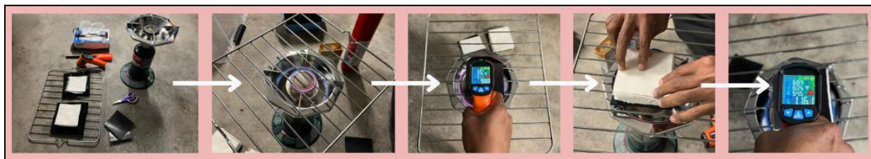
Fig 7: Materials and basic procedure of Fourier's Open Flame Test
