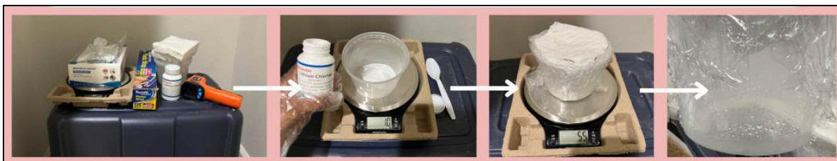
Fig 8: Materials and basic procedure of Moisture Vapor Transfer Rate (MVTR) Test
